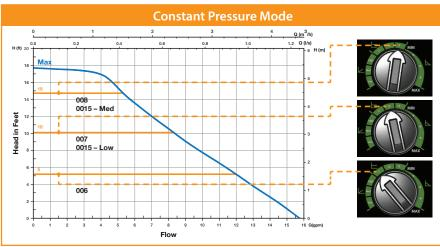
In constant pressure mode, the circulator maintains a constant pressure differential ( $\Delta p$ -c) in the system as heating load increases or decreases. Selection options are 5, 10, or 15 feet of head constant pressure.
