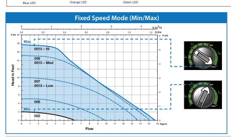
Fixed speed mode allows the installer to fine tune the circulator flow rate to precisely match design load conditions. It is infinitely variable between min/max settings.
