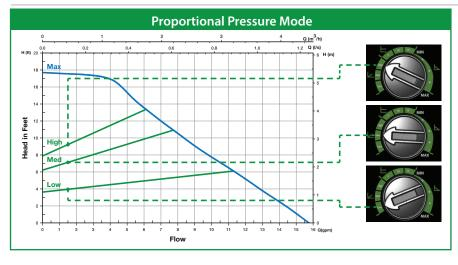
In proportional pressure mode, the circulator maintains a proportional pressure differential ( $\Delta p$ -v) in the system as heating load increases or decreases. Flow will change in relationship to the change in pressure differential.
